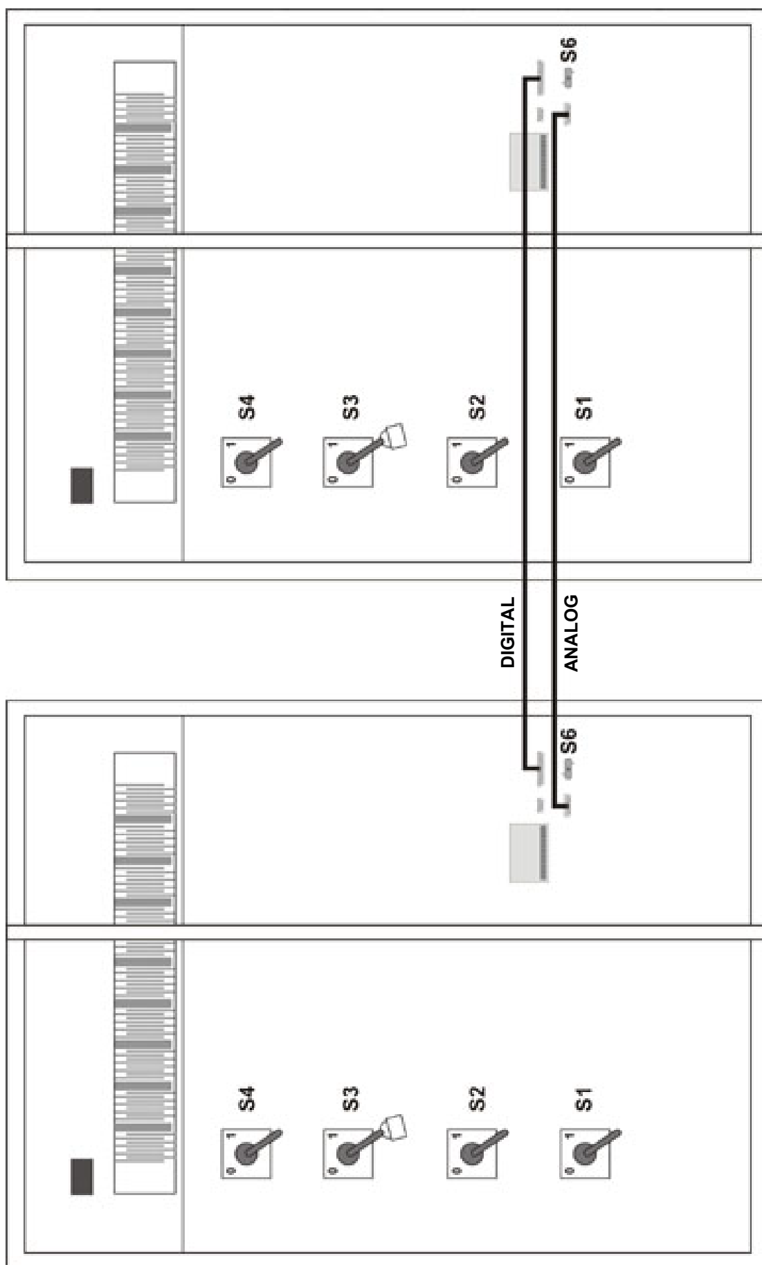
Figure 6-4-e Switch and Fuse Positions and Signal cable connections for parallel operation (100-120-160-200 kVA)
